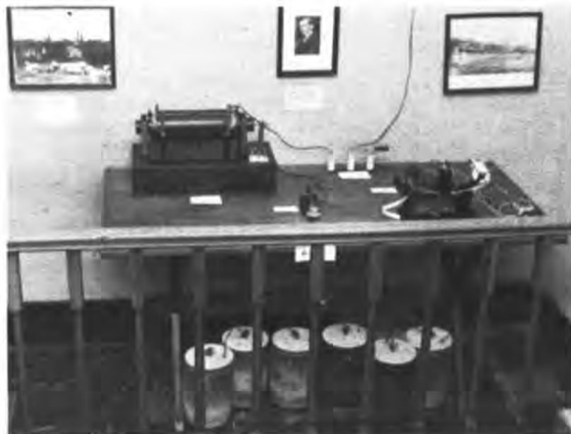
Replica of the original Marconi equipment of the wireless station at Twin Lights, NJ. This rig, without tuning or coupling, no doubt radiated on every wavelength in the spectrum. Such gear is strictly illegal today.
